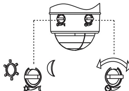
After adjusting the TIME and LUX settings, rotate the motion sensor dome to the left and align the arrows on the lamp housing and the motion sensor dome.
