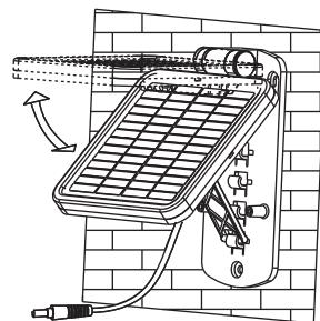
3. Carefully route the solar panel cable to the light fixture. Plug the solar panel cable into the connector extending from the bottom of the battery case.
