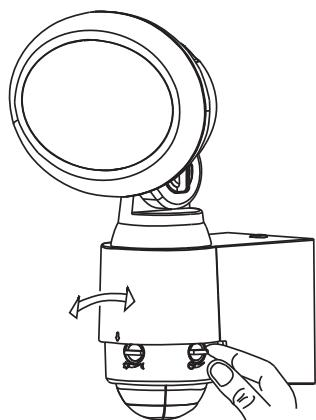
**TIME — Duration Time:** The duration time will adjust from 10 seconds to 1 minute, depending on how long you wish the unit to stay on after motion is detected. Note: Once the light has been triggered, any additional motion detection will start the timed period again from the beginning. Turn the TIME dial counterclockwise to increase the duration. Turn the TIME dial clockwise to decrease the duration.
